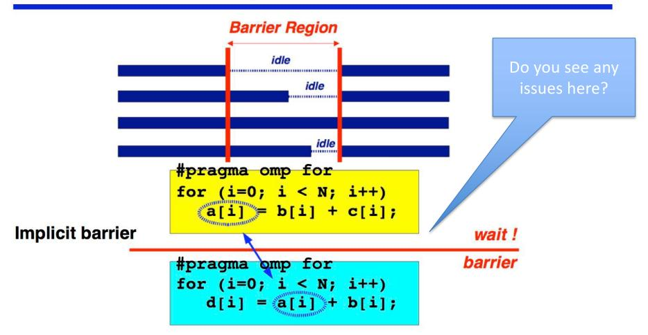
NOTE: barrier is redundant if there is a guarantee that the mapping of iterations onto threads is identical in both loops
