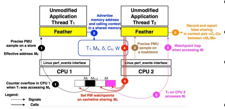
Debug registers enable trapping CPU execution for debugging when the PC (program counter) reaches an address (breakpoint) or an instruction accesses a designated address (watchpoint)
